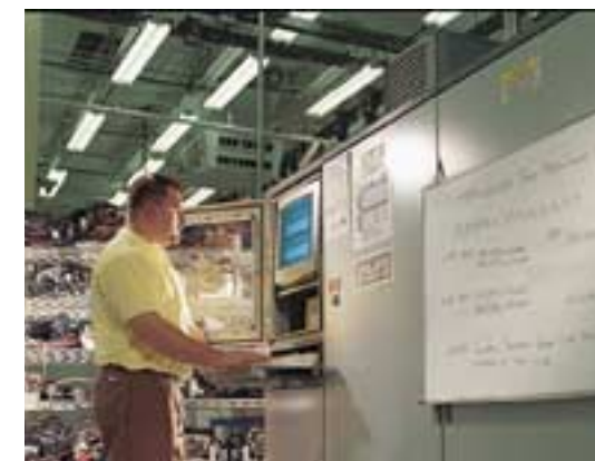
As part of the design and testing process, Bussed Electrical Centers are cycled to simulate vehicle operation.
