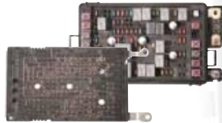
Routed wire electrical center
